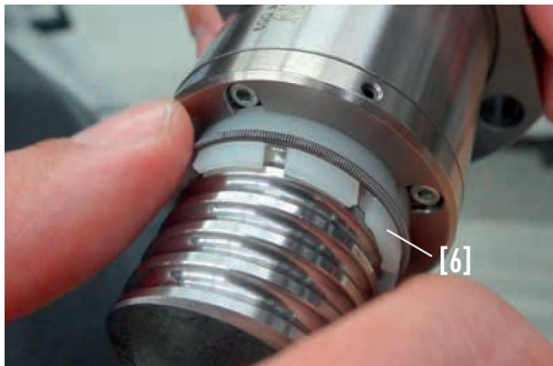
Fig. 4.15: Removing the finger wiper
