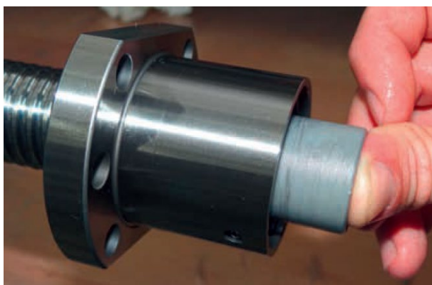
Fig. 4.11: Disassembling the nut using an assembly sleeve
