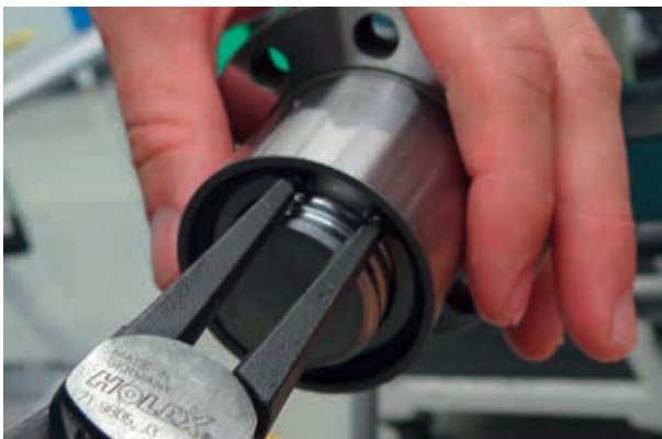
Fig. 4.9: Removing the circlip
