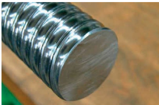
Fig. 4.3: Shaft end before assembling the NBR wiper
