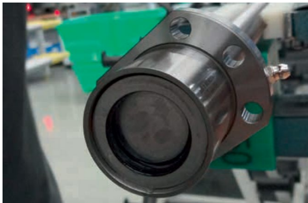
Fig. 4.10: Removing the metal ring
