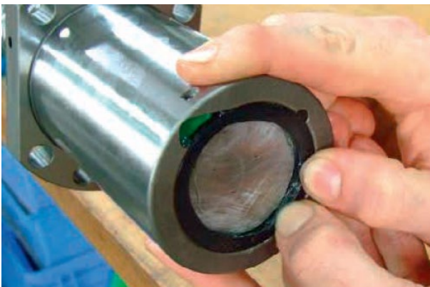
Fig. 4.7: Fixing the wiper while slowly screwing the nut onto the shaft
